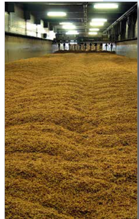
Classic Saladin boxes with turner-stripper guarantee uniform germination.
